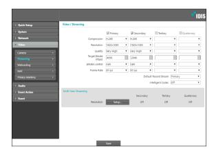
Primary/Secondary/Tertiary/Quaternary(priority: Primary > Secondary > Tertiary > Quaternary The lower stream settings may change depending on higher stream settings. The tertiary and quaternary streams may not be available depending on higher stream settings. (refer to the table below).
